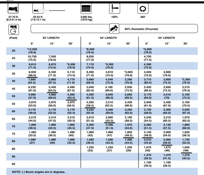
\*This capacity is based upon maximum boom angle.
