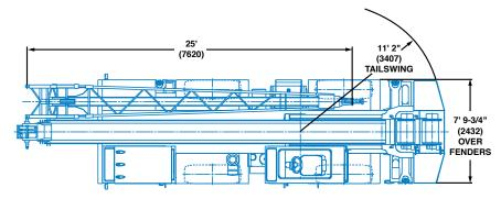
TURNING RADIUS - (2 Wheel Steer) 29' 6" (9029) (4 Wheel Steer) 20' 3" (6166)
